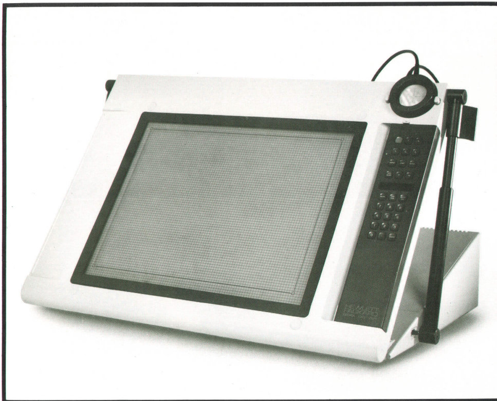
Fig. 1. Model 9874A is an advanced microprocessor-controlled digitizer that provides 25- \mu\text{m} resolution and \pm 125\text{-}\mu\text{m} accuracy. Its adjustable glass platen accommodates a variety of media. The keypad helps the operator control the digitizer/computer system.
